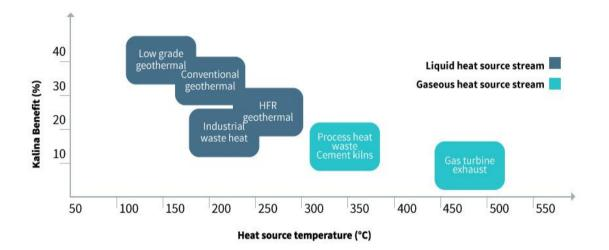
The KALiNA Cycle<sup>®</sup> has application in a wide range of industrial and renewable energy sectors. These have been divided into two key areas – industrial energy efficiency and renewable energy generation. The Industrial Energy Efficiency sources heat generated as a by-product or waste from an existing industrial process, including power generation. The Renewable Energy Generation is based on heat from a renewable source, for example, geothermal groundwater or solar thermal applications.
